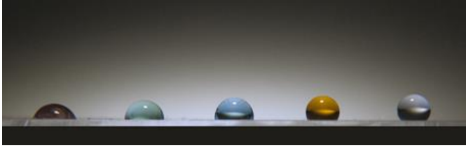
Figure 2. Schematic illustration of droplets of identical volume displaying gradually decreasing contact angles due to the surface energy gradient.
